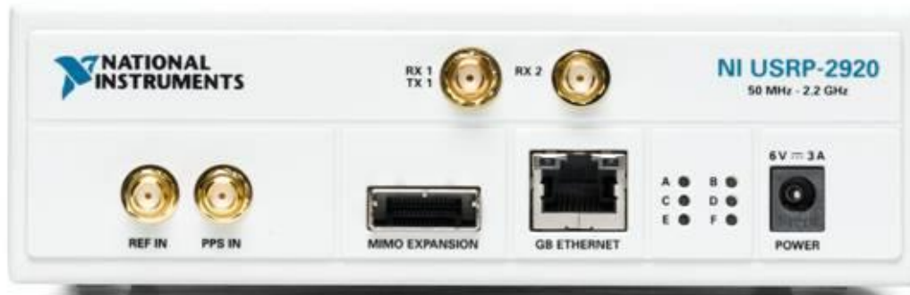
Figura 8. USRP 2920. Fuente: National Instruments.
