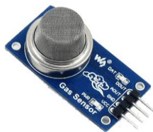
Figura 7 Sensor de gas MQ-2
